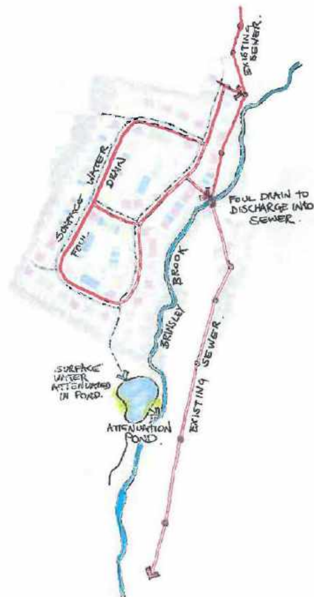
Drainage Diagram showing the SuDs and foul drainage system
