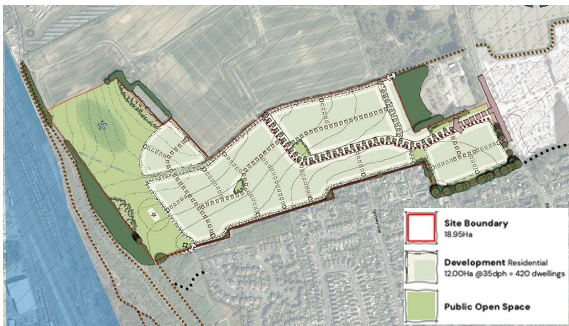
Figure 2: Extract of 'Illustrative Masterplan' Drawing No. P23_2377_DE_O14 and Key. (Rail Land at Toton Sidings indicatively shaded blue by Firstplan)
